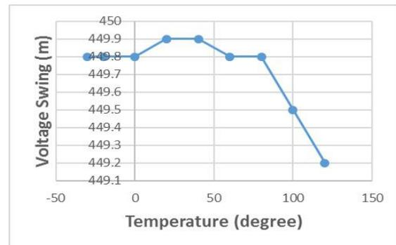
Fig. 14. Variation of voltage swing (m) with temperature.
