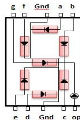
Fig. 1. Diode connections.
