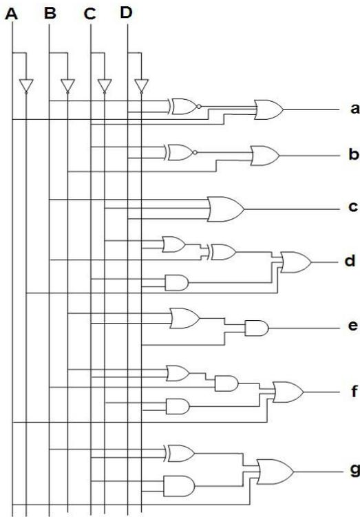
Fig. 2. Schematic of 7-segment display.
