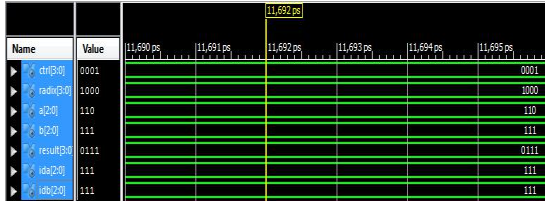
Fig. 5. Simulated waveform for OR operation.
