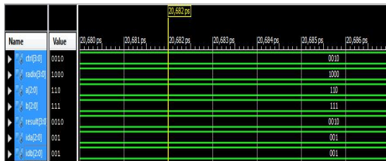
Fig. 6. Simulated waveform for NAND operation.
