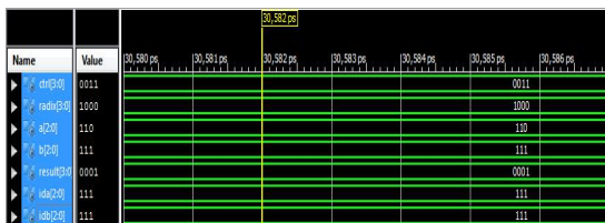
Fig. 7. Simulated waveform for NOR operation.
