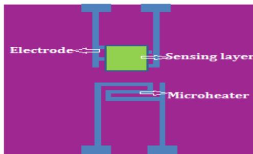
Fig. 1. Different parts of gas sensor.
