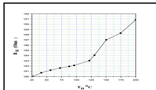
Fig. 7. Microheater resistance ( $R_H$ ) as a function of microheater temperature ( $T_H$ ) at 27°C ambient temperature.
