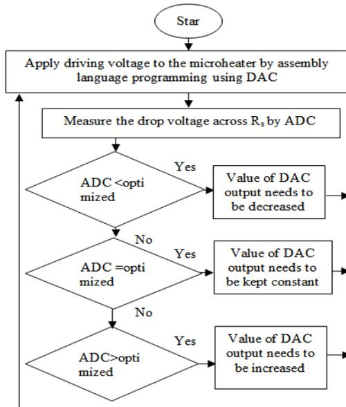
Fig. 10. Flow chart showing compensation technique.
