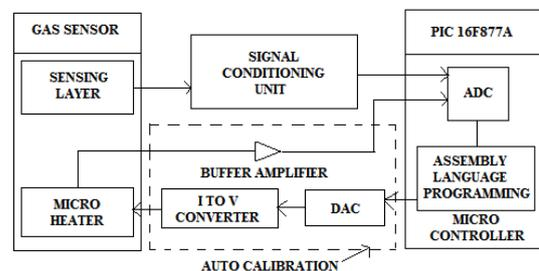
Fig. 2. Schematic of interface circuit designed for gas sensor.
