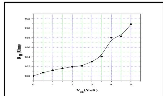
Fig. 6. Microheater resistance ( $R_H$ ) as a function of microheater voltage ( $V_H$ ) at 27°C ambient temperature.
