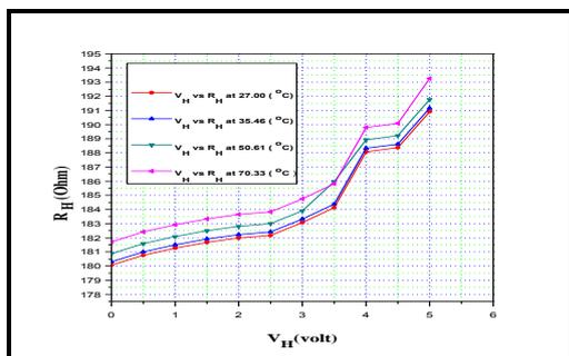
Fig. 8. Effect of ambient temperature on microheater resistance  $R_H$ : curves at 27°C, 35.46°C, 50.61°C and 70.33°C.
