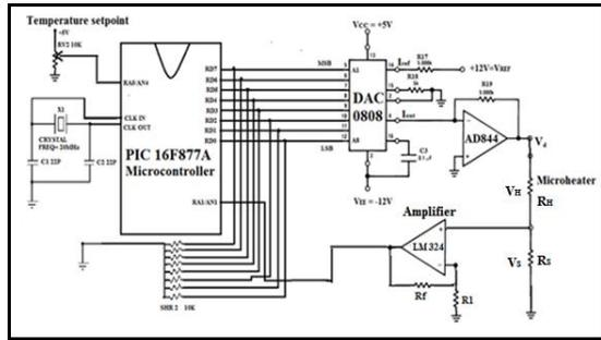
Fig. 3. Microheater temperature control circuit.
