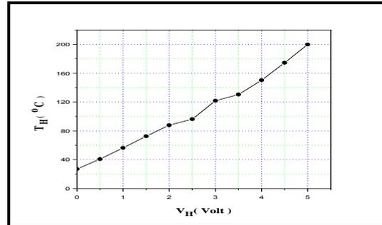
Fig. 5. Microheater temperature ( $T_H$ ) as a function of microheater voltage ( $V_H$ ) at 27°C ambient temperature.
