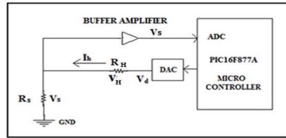
Fig. 9. Schematic circuit for compensating the ambient temperature.
